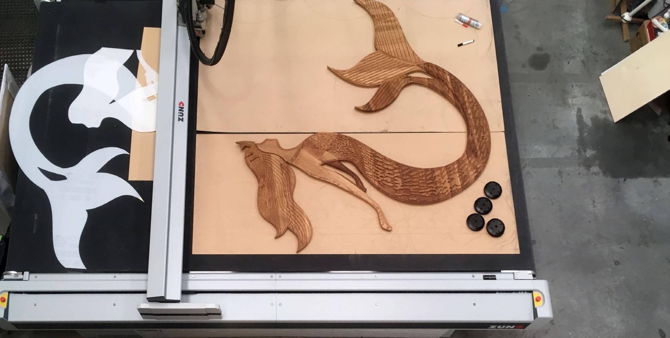
Fabrication of a reclaimed oak wall feature on a Zund multi-material cnc machine.
